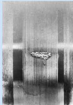
More advanced spalling
