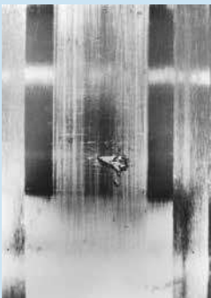
Early fatigue spalling
