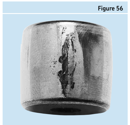
Corrosion on roller surface caused by water in lubricant while bearing was standing still
