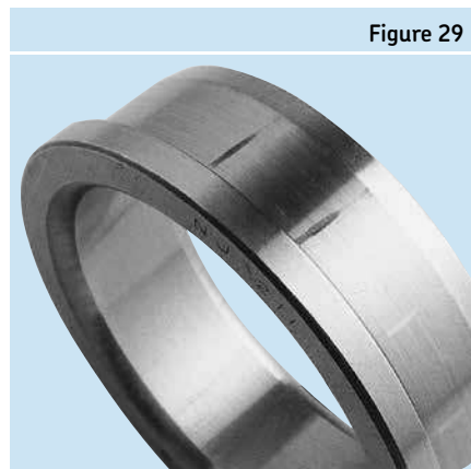
Smearing caused by excessive force in mounting
