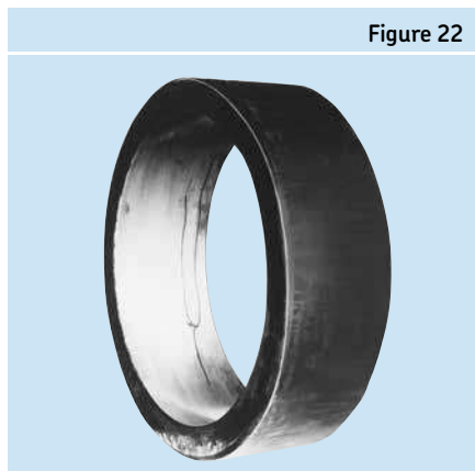
Cracks caused by faulty housing fit
