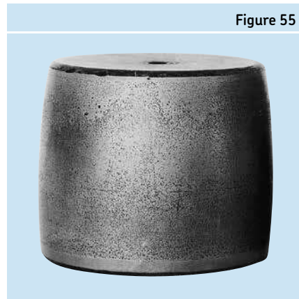
Corrosion of roller surface caused by formation of acids in lubrication with some moisture present
