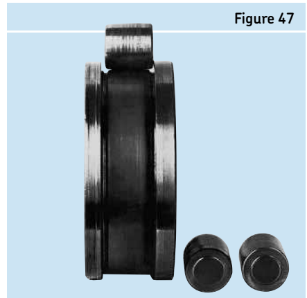
Grooves caused by wear due to inadequate lubrication
